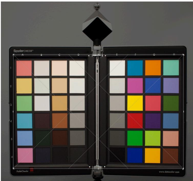
Cropping is done with Lightroom or ACR's crop tool. Crop to the four white dots just outside of the patch area. Use the rotate function of the crop tool to straighten the target image. Activating Lightroom 3's lens profile function will reduce lens distortion in your target shot, but this is not really necessary.
