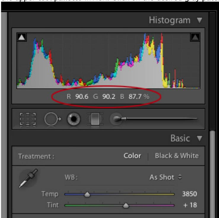
Next look at RGB values or Percentages of the White patch (E1). Adjust the exposure slider until the white patch lists as approximately 90% in Lightroom, or about RGB 230, 230, 230 in ACR. Next check the black (E6). The Blacks adjustment (or in some cases the Shadows adjustment) is used to set the black value to 4% in Lightroom, or RGB 10, 10, 10 in ACR. If the value is below this level, it may be best to leave it as shot, or reshoot with brighter illumination.
